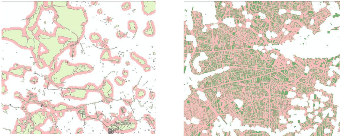
Figure 4. Preliminary generalisation results for polygon data. Green areas represent the original geometries; red areas represent the expanded (first image) or condensed areas (second image). Pictures are adjusted to a presentation scale of 1:300.000.
