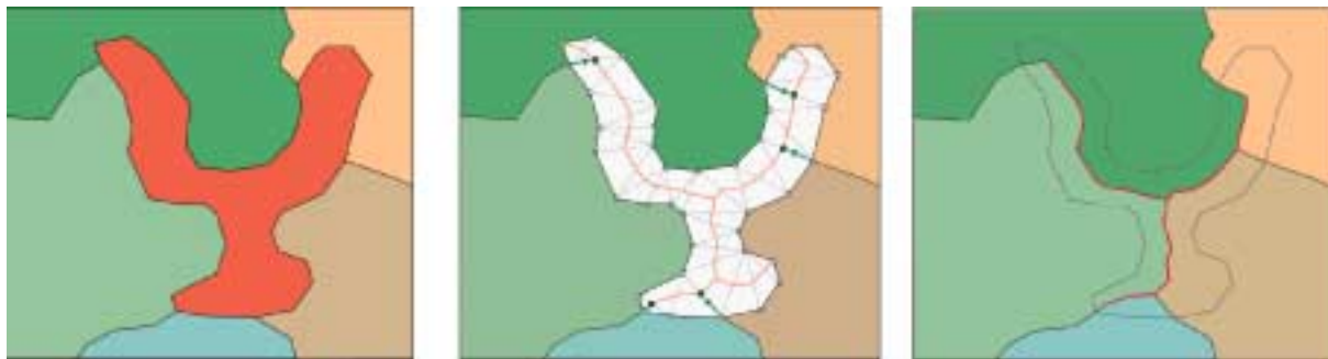
Figure 2: Algorithm proposed by Bader (1997) for eliminating a polygon based on the construction of a skeleton of the object (Source: Bader 1997).
