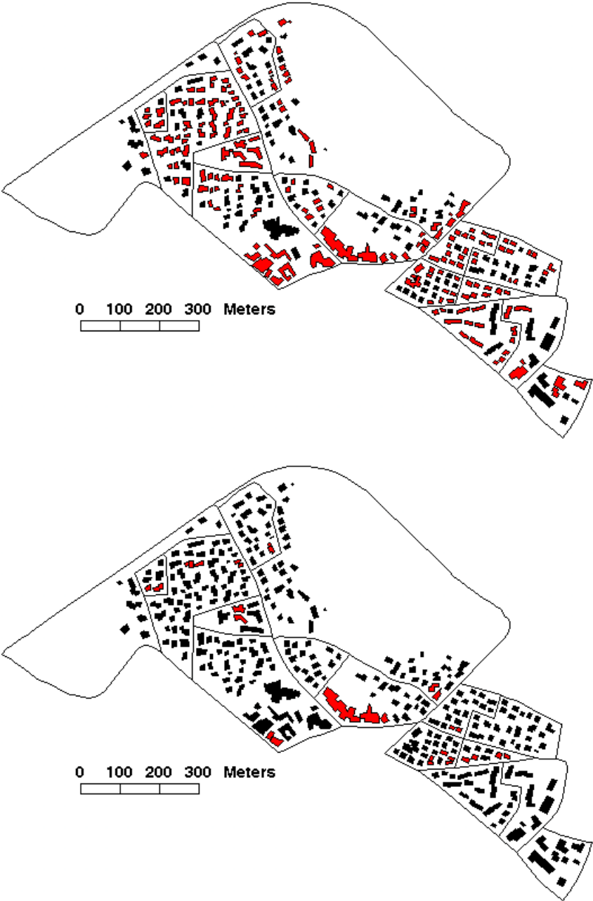
Figure 3. BDTopo data before (top) and after (bottom) application of simulated annealing algorithm Objects shown in red are involved in spatial conflict of some kind.
