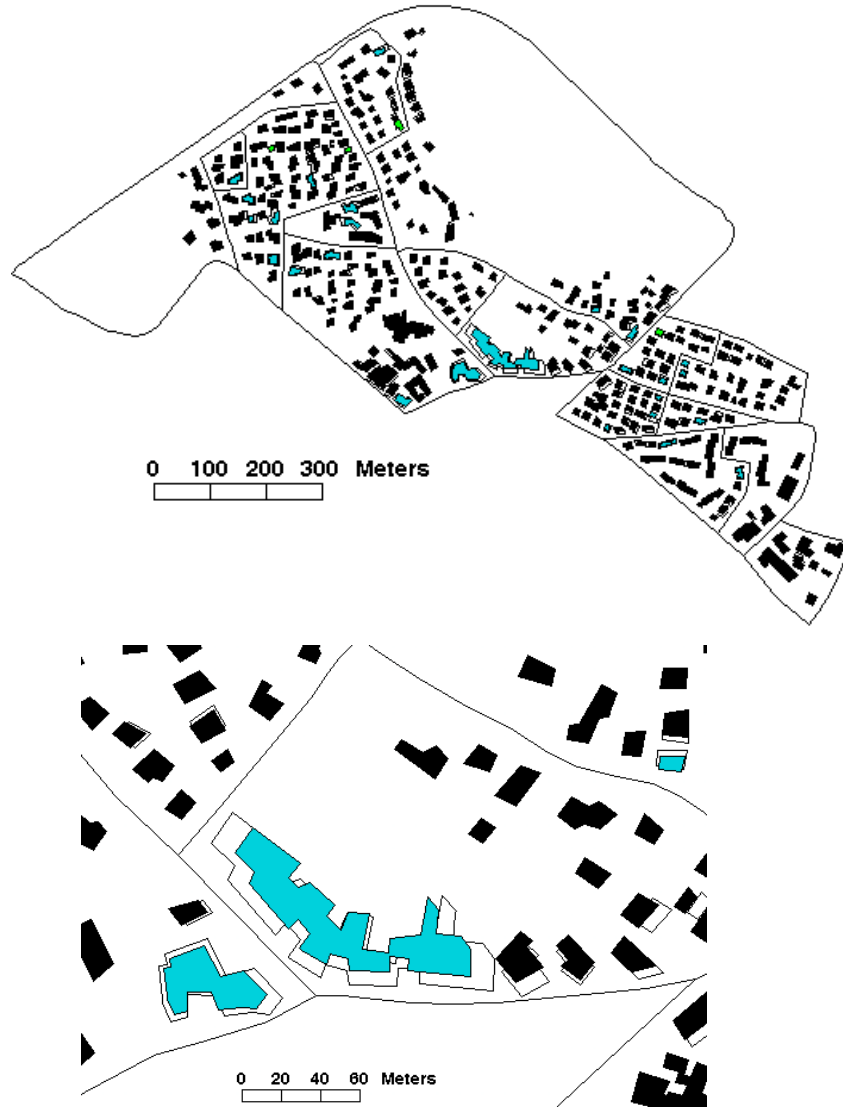
Figure 7. Full and zoomed-in version of display obtained using object displacement, reduction, enlargement and deletion. Reduced objects shown in blue (no object enlargement required).
