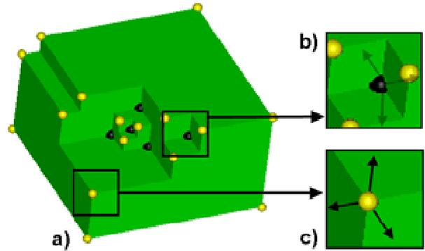
Figure 5. a) Fully convex (yellow) and fully concave (black) vertices, determined by computation of coedge-extension: b) all end points of extended edges inside  $\Rightarrow$  fully concave vertex, c) all end points outside  $\Rightarrow$  fully convex vertex
