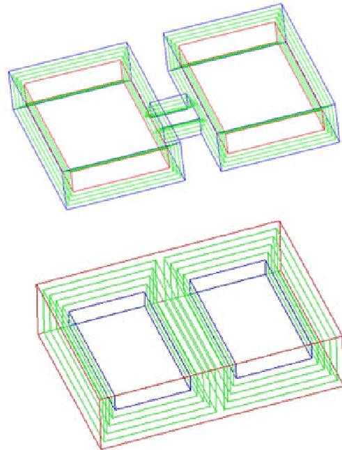
Figure 3. Split (top) and merge (bottom) for erosion and dilation in 3D: blue - original object; green - incremental steps; red - resulting object.
