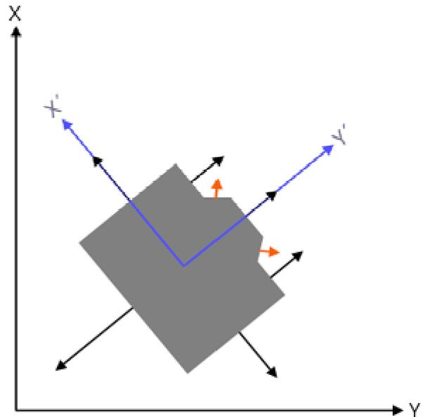
Figure 13. View from the top: X, Y: World coordinate system; X', Y': Local coordinate system; Black arrows: wall-facets parallel to main directions; Red arrows: wall-facets deviating from main directions
