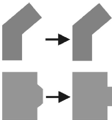
Figure 12. Strong inclinations have to be preserved for large structures (top), whereas small parts need to be squared (bottom)
