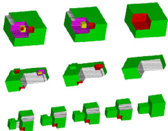
Figure 7. Results for the detection and elimination of stair- / step- and box-structures (several LODs)
