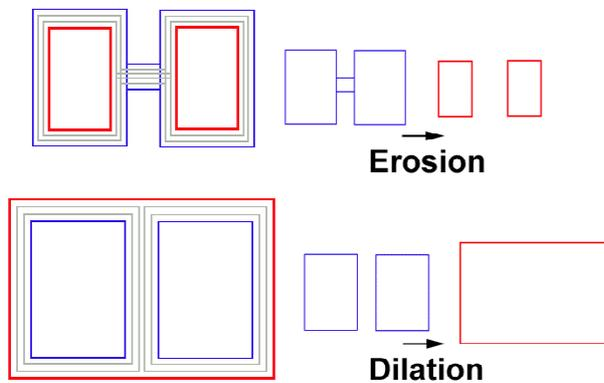
Figure 2. Mathematical morphology applied to vector data - split (top) for erosion; merge for dilation (bottom)
