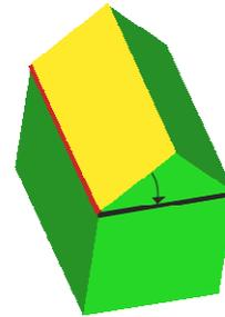
Figure 9. The roof-facet (yellow) is rotated (tapered) around the eave-line (red) until the roof-facet becomes horizontal.
