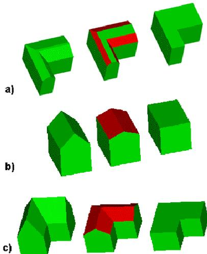
Figure 8. Results for removing inclined roof-structures by means of tapering
