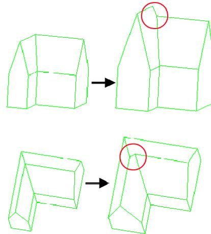
Figure 10. Differently inclined roof-facets can lead to unsatisfactory results when tapering, because no unique intersection point exists due to different heights.
