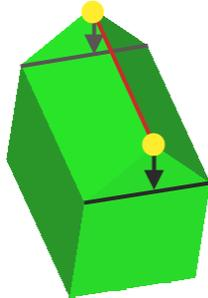
Figure 11. Movement of vertices: The vertices of the ridge are shifted downwards until they have the same height as the eaves.
