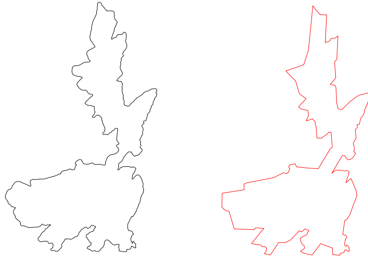
Figure 8. Peristera Island coastline (left) and its 153 critical points connected with line segments (right).
