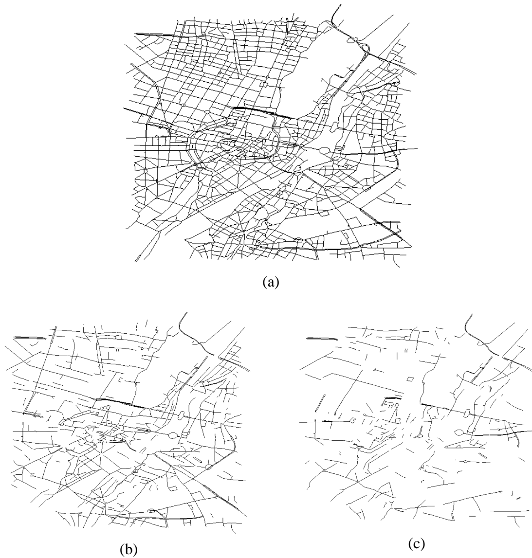
Figure 5: The original network (a) and the selected streets at the level of 50% (b) and 25% (c) based on k-means algorithm
