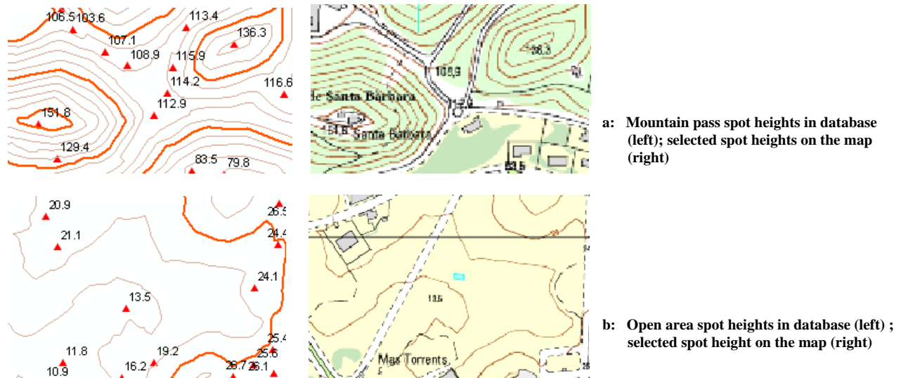
Figure 5: Spot height selection in terrain context - (thanks to the Institut Cartogràfic de Catalunya for the data)
