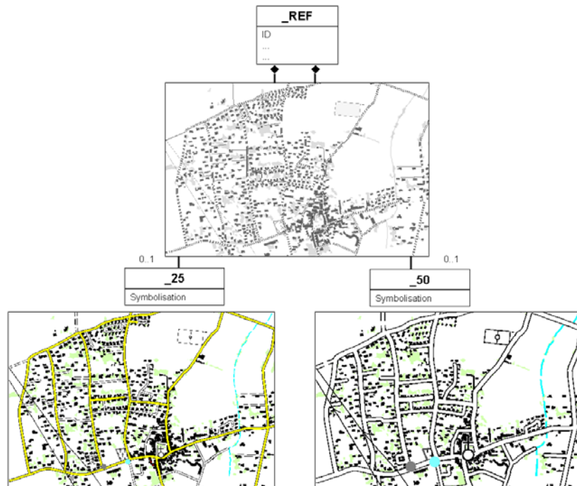
Figure 10 - Precoding of the DCM 25k-50k, with network removal concerning the 50k (Application with Lamps2)
