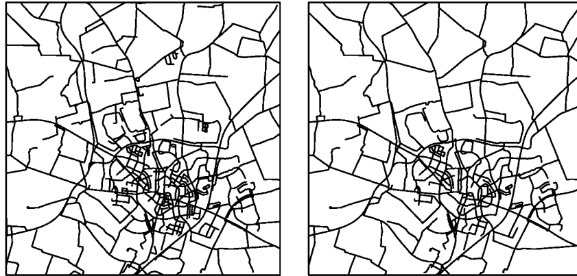
Figure 3 Generalized road network with 25% (left) and 35% (right) reduction of length. ©Lantmäteriverket 2004. From GSD-Property Map reference no. M2004/2828
