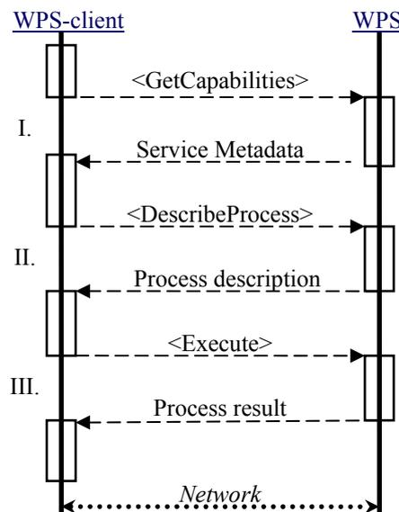
Figure 2. Basic client-service communication
