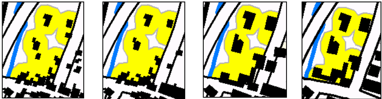
a) Initial data b) After elimination c) After micro generalisation d) After displacement
