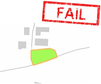
Perimeter p = 119,4 mArea  $a = 827.7 \text{ m}^2$ Virtual Radius *vr* = 18 m Circularity ratio *cr* = 7.25
