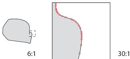
Figure 4: A cubic Bezier curve of a polygon, broken down into polyline segments
