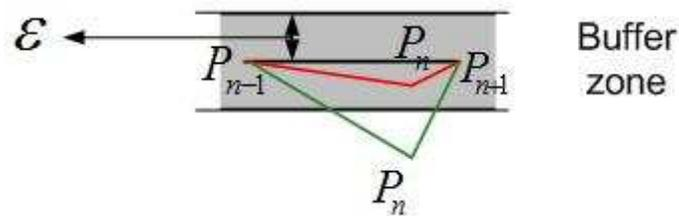
Fig.2. Removing the point located inside of the buffer zone, whereby the width of the buffer zone  $2 \cdot \varepsilon$  can be predefined for the given data.
