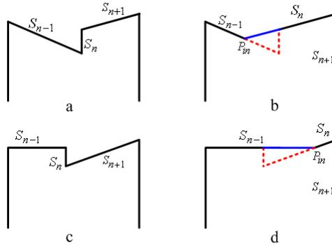
**Fig.6.** The shortest side is removed by intersecting its flanking neighbors
