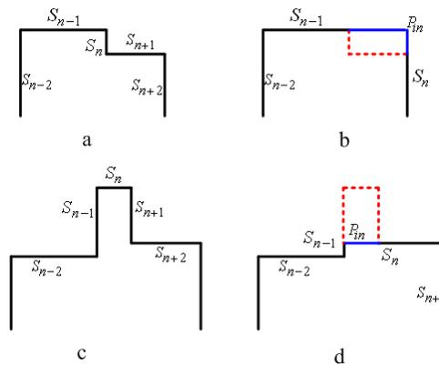
**Fig.5.** Different parts of a ground plan a) and c) and their simplification results b) and d) after the first iteration
