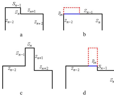
**Fig.4.** Different parts of a ground plan a) and c) and their simplification results b) and d) after the first iteration
