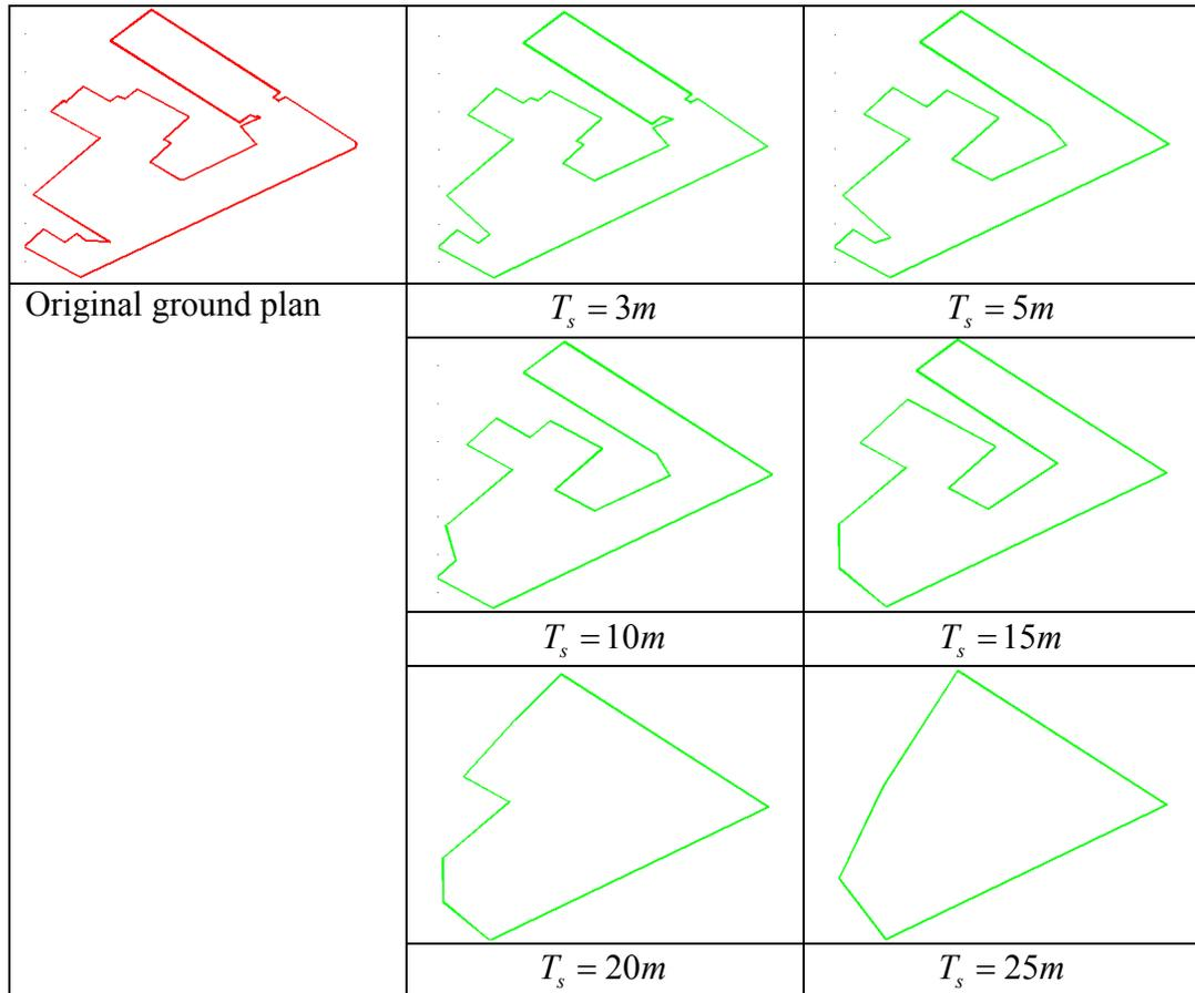
Fig.10. A building with a complex geometric form and the simplification results with different thresholds
