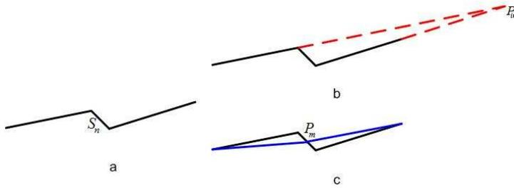
**Fig.8.** Removal of a sharp angle caused by removal of a short side
