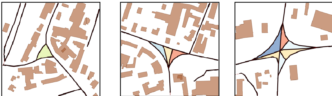
Figure 3: road junctions are detected using road cycles. Each road junction can be formed by more than one road cycle
