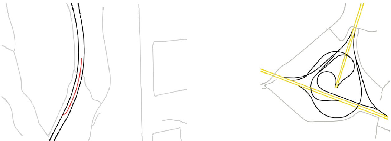
Figure 10: (left) an error in the classification of the input data is detected: the edge classified as highway (red) is too short to be a highway and, as a slip road, it is not connected to anything; it will then not be considered part of the highway. (right) The classification of slip roads and carriageways is reliable also in complex cases.
