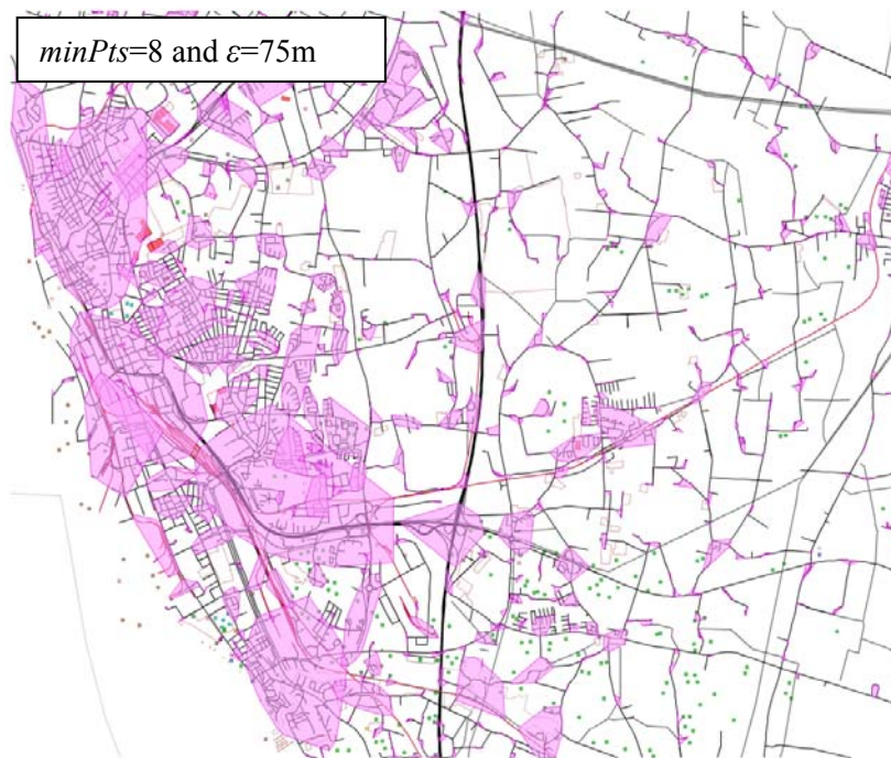
Figure 6. Clusters created with \text{minPts}=8 and \epsilon=75\text{m} . Max length of line segments is 200 m.
