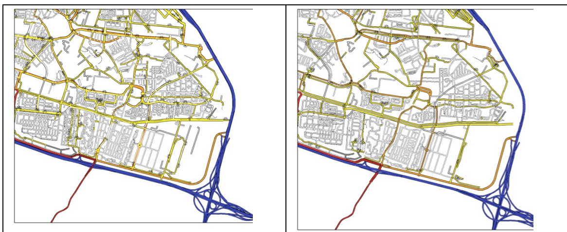
Figure 2 Thinning of the road network before (left) and after (right) generalisation (displayed with same symbol size and at same scale)
