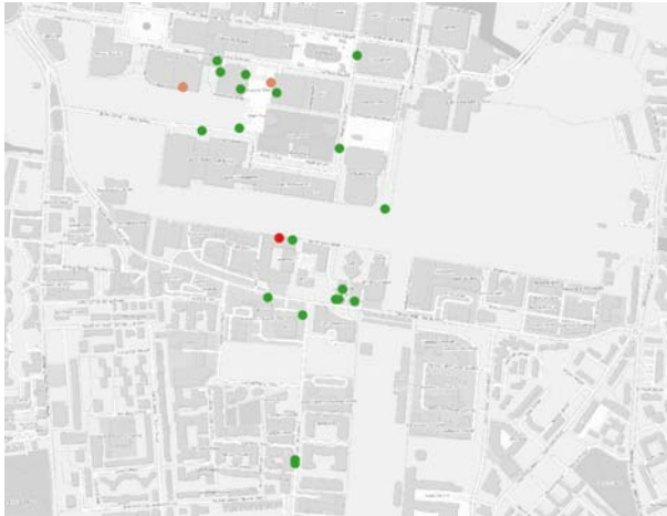
Figure 4 - A classic selection operation where features are selected based directly on a given classification attribute (amenity=restaurant in this case) or ranking attribute. Selected features shown in orange.
